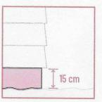
Create a 15 cm ground-tosiding non-combustible clearance (e.g., install cement board or metal skirting).
