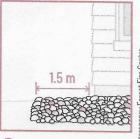
Install non-combustible ground surfaces within 1.5 m of the house (mineral soil, rock, concrete or stone).
