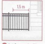
Install non-combustible fencing within 1.5 m of the house (cement fiber, metal, chain link or stone).
