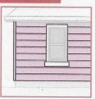
Install non-combustible siding (stucco, metal, stone, cement fibre board).
